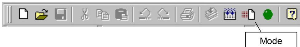
Mode button puts the board into **Run** or **Program** mode. In Run mode, the micro-controller is executing the program in its memory. In Program mode, the micro-controller is in Reset state so no programs are running. In Program mode, micro-controller's flash memory can be changed and a new program can be downloaded.
